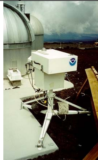
Brewer instrument which measures "Total Ozone"
